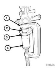
5. Position suitable tool as shown to remove lower ball stud.
