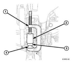
4. Position suitable tool as shown to remove upper ball joint.
