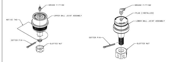
CAUTION: Replace any worn or damaged steering knuckle and axle components prior to replacing ball joints.
