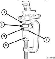
suitable tool as shown to install lower ball joint.
