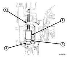
suitable tool as shown to install upper ball joint.
